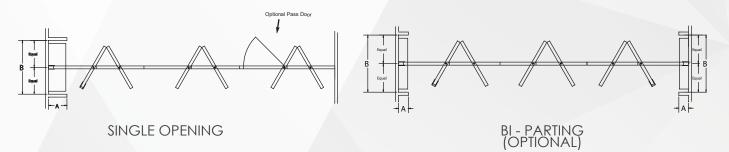
Select for wall-to-wall space division. Panels are hinged in pairs allowing fast setup. They may be stacked at either or both ends of the track or in a "pocket". One or more pair of panels may be placed anywhere along the track for use as sight dividers.
